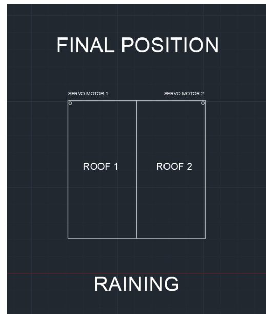
Fig. 16: Final Position of the Roof (Servo motors at 90 degree)
